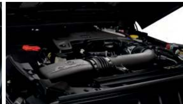
Cold Air Intake System 18
