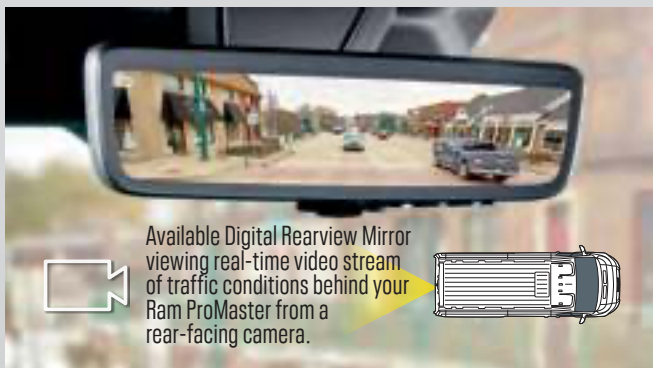
AVAILABLE DIGITAL REARVIEW MIRROR The available Digital Rearview Mirror replaces a traditional reflective rearview mirror with a 9.2-inch-wide LCD monitor that displays real-time video from a rear-facing camera. The camera is located on the back of the van, so the view is unobstructed. Unlike back-up cameras, the vehicle doesn't need to be in Reverse to activate, and the view is a high resolution.
