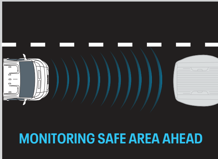
STANDARD FULL-SPEED FORWARD COLLISION WARNING PLUS (FSFCW+) WITH PEDESTRIAN/CYCLIST EMERGENCY BRAKING 15 The standard FSFCW+ 15 system provides both audible and visual warnings to alert the driver when it detects a potential frontal collision. The warnings are intended to help provide the driver with enough time to react to, avoid or mitigate a potential collision.
